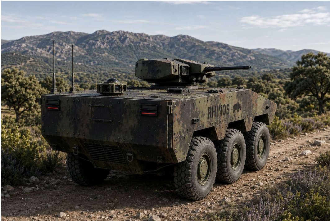
Rendering of RHINOS COMBAT, the heavy 6x6 fire support UGV of the RHINOS family. Credit: Miriad Global
